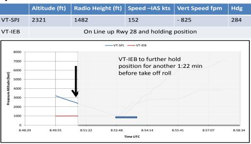
The active runway was occupied by VT-IEB holding at lineup from 'C' intersection while VT-SPJ continued its approach and was advised to expect landing clearance at short final. The CVR of VT-SPJ has recordings to infer that it was being apprehended by this crew that ATC is pushing them into very tight situation and the Go Around procedure was also reviewed by them.
